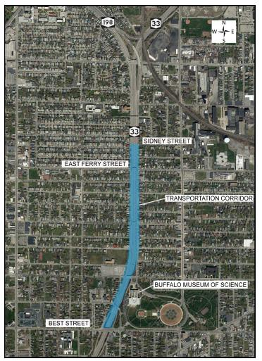
Figure 1: Proposed Tunnel Location The project comprises of an approx. 4,150 ft long, 2 x 3 lane lid
