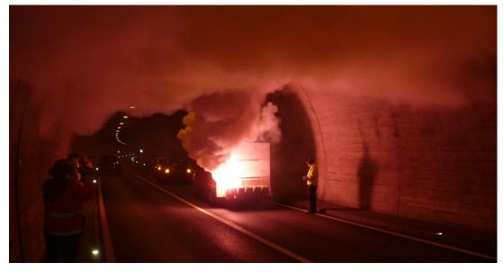
Figure 15: Hot smoke Test in a Road Tunnel
