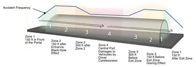
Figure 3: Tunnel Zones with Expected accident Frequency
