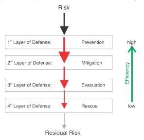
Figure 4: Priorities / Layers of a Defense of a Four-Stage Safety Concept
