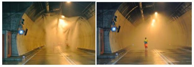
Figure 11: Test Activation of Water Mist FFFS in a Road Tunnel
