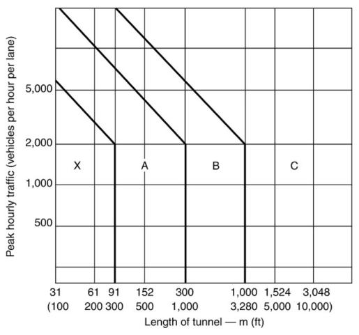
Figure 6: Tunnel Categories According to NFPA 502
